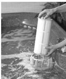
1) Center filter cartridge over canister
